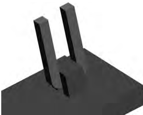
Fig. 71 Three-dimensional computer model of heating selected areas of a plate by using a hairpin inductor. Courtesy of Infolytica Corp.
