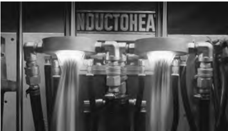
Fig. 50 Induction dual-scan hardening uses spray quenching. Courtesy of Inductoheat, Inc.
