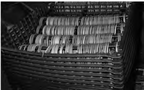
Fig. 33 Flat rings for tempering, case study 3
