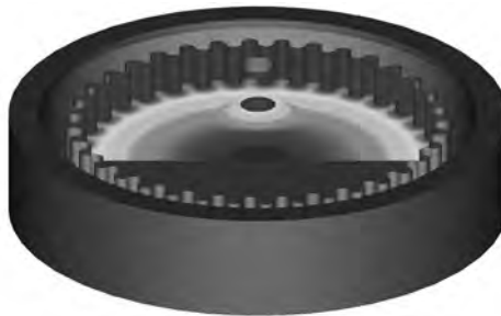
Fig. 70 Three-dimensional computer model of current density distribution when heating the inside diameter of a gear. Courtesy of Integrated Engineering Software, Inc.
