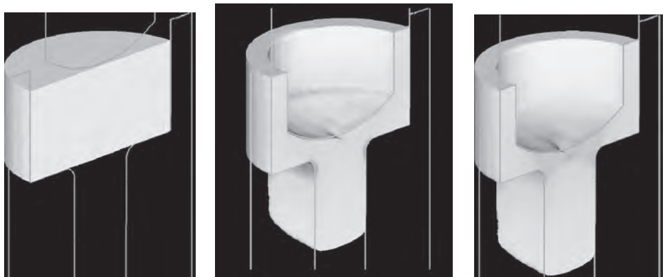
Fig. 36 Predicted geometry at different stages of the extrusion process
