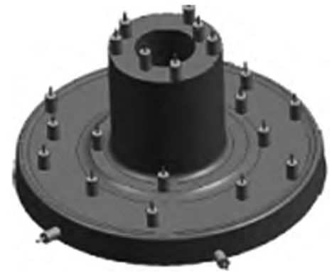
Fig. 12 Heat-transfer coefficient measurement using a disk outfitted with thermocouples
