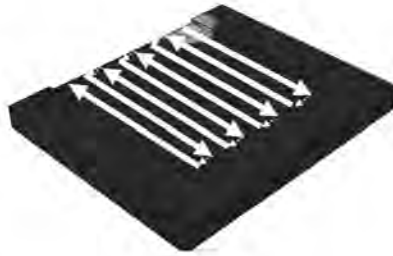
Fig. 10 Process parameters and deposit sequence for scour repair on a thin plate
