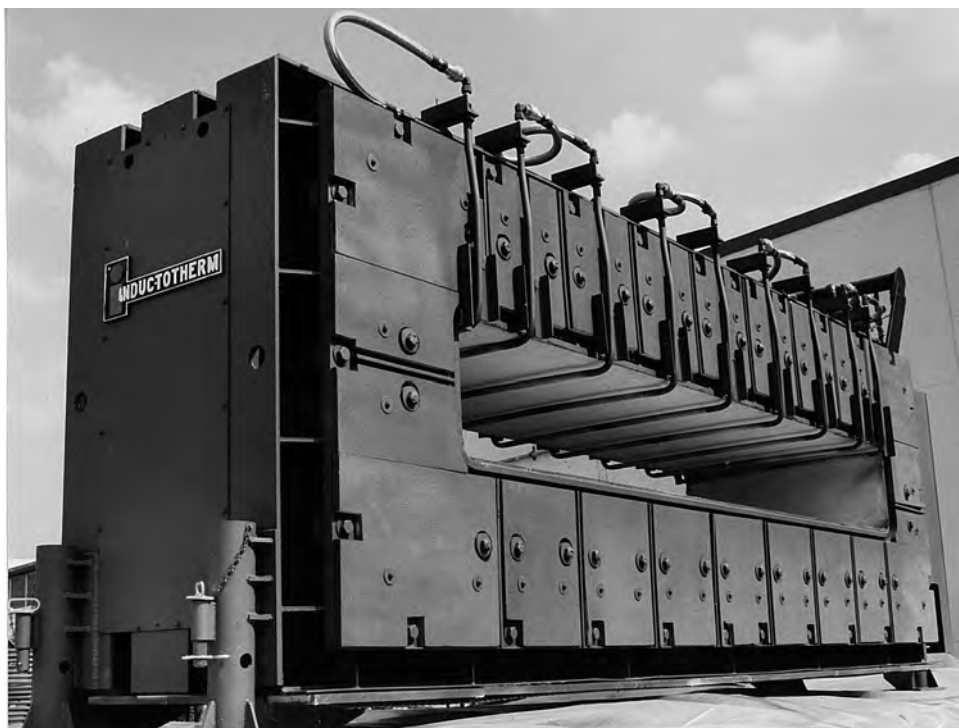
Fig. 35 Unique 6000 kW/110 Hz induction coil provides heating of the world's largest steel slab. Slab geometry: 3.2 m wide and 0.22 m thick. Courtesy of Inductotherm Corp.
