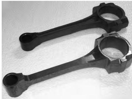
Fig. 12 Pressed-and-sintered preform (foreground) and powder-forged connecting rod
