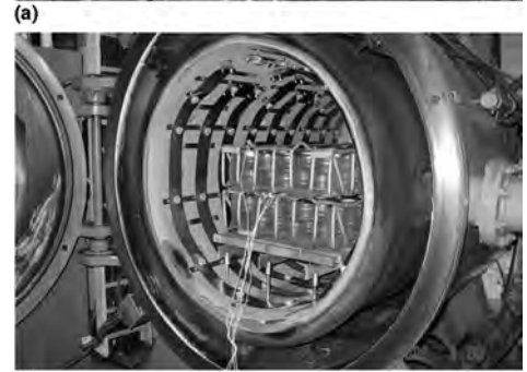
Fig. 31 Load pattern and arrangement of thermocouples
