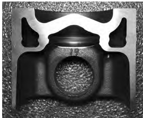
Fig. 40 Spinduction produces welds at very low rotational velocities with minimal flash projection. Source: Ref 29
