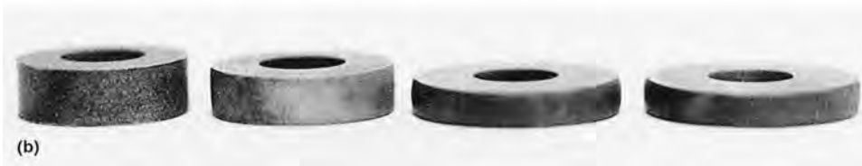
Fig. 10 The ring test. (a) Schematic of metal flow. (b) Example rings upset to various reductions in height
