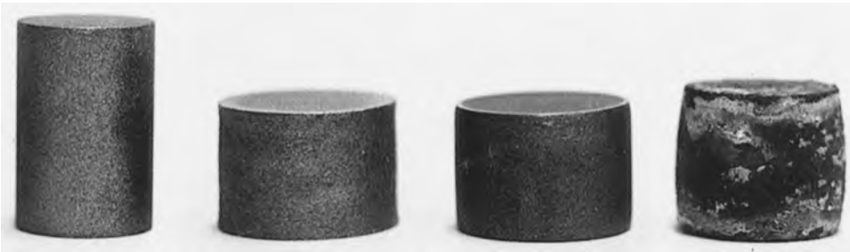
Fig. 8 Left to right, specimen before compression and AISI 1018 steel, nickel alloy 718, and Ti-6Al-4V after hot deformation
