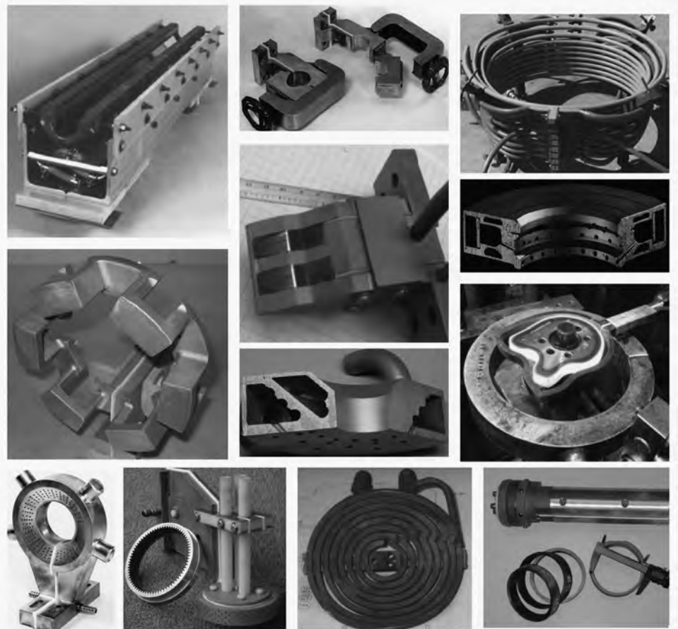
Fig. 4 Variety of inductors for various induction heat treating applications. Courtesy of Inductoheat, Inc.
