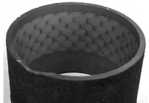
Fig. 77 Snakeskin hardness pattern. Source: Ref 1
