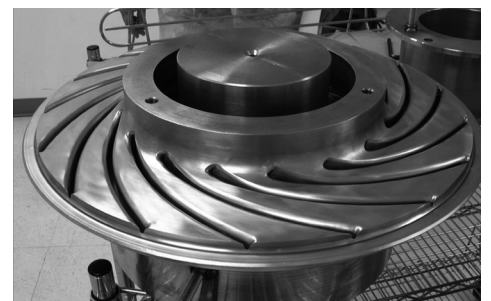
Fig. 4 Capsule and insert for hot isostatic pressing of a net shape impeller
