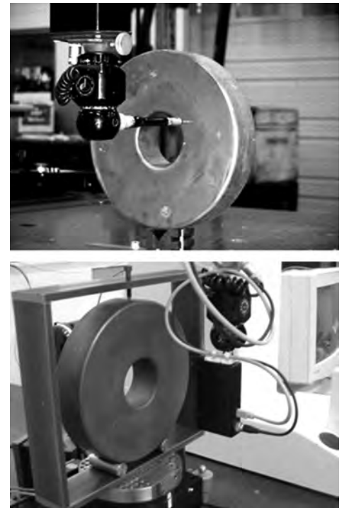
Fig. 16 Coordinate measurement machine inspection and optical scanning setup for measuring distortions
