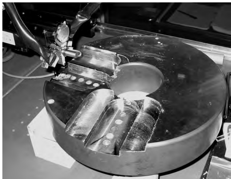
Fig. 18 Machining of slots during measurement of residual stresses
