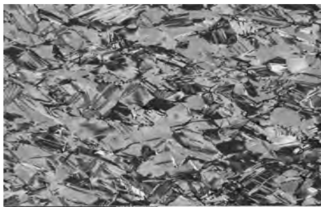
Fig. 8 Example of an orientation map of a lightly deformed titanium showing a high density of deformation twins. Courtesy of Nathalie Bozzolo
