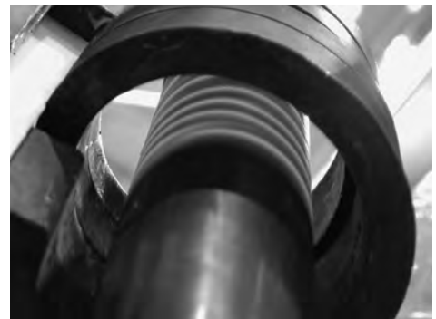
Fig. 78 Multiple stripes appear due to a striping phenomenon. (Note that the induction coil has only four turns.) Source: Ref 121
