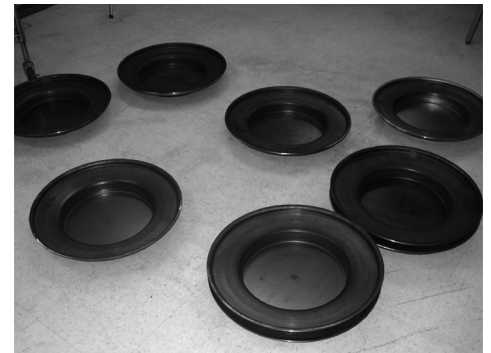
Fig. 3 Capsule elements for hot isostatic pressing of a blank for a turbine disk
