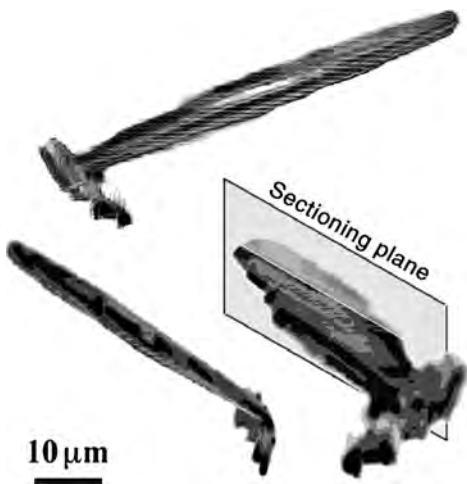
Fig. 6 Three perspective views of the Widmanstätten cementite precipitate indicated by an arrow in Fig. 5. Source: Ref 13
