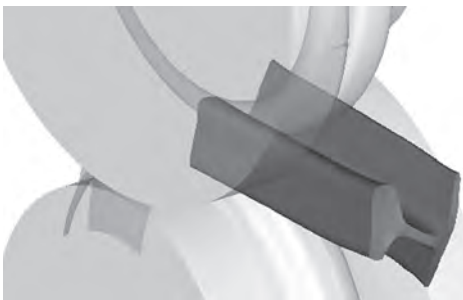
Fig. 6 Rail section exiting the fourth-from-last pass
