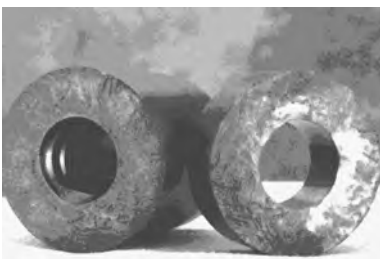
Fig. 54 The failure mode of the die insert in the first station was a low-cycle fatigue fracture, as shown
