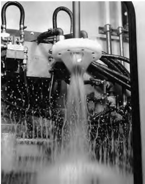
Fig. 1 Induction scan hardening requires rapid cooling. Courtesy of Inductoheat, Inc.
