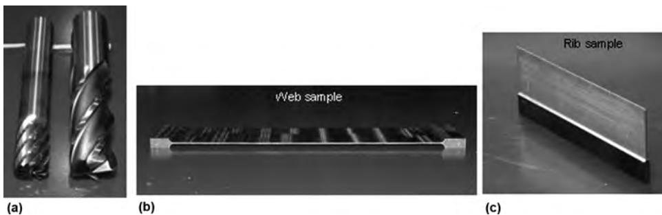
Fig. 35 (a) Tungsten carbide and AISI M-42 cutting tools. (b) Machining of subscale webs. (c) Machining of subscale ribs
