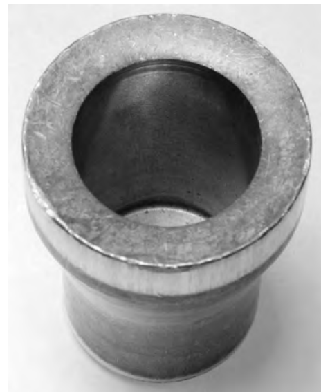
Fig. 53 After the redesign, the inside diameter is free of defects
