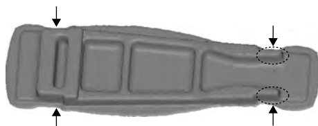
Fig. 77 Simulation result using the initial preform design/deformed shape
