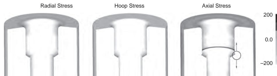
Fig. 56 The component stresses were evaluated on the original design to isolate the root cause of the failure. The dark colors represent tension and the light colors compression. Hoop and radial stresses (light color) are essentially compressive. The circle highlights a tensile stress in the axial direction, as shown with the arrows
