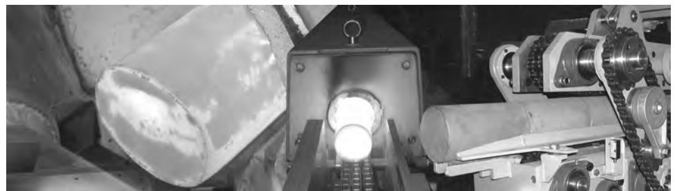
Fig. 1 Billets or bars are fully or partially heated in cut lengths or continuously and are forged in presses, hammers, or upsetters
