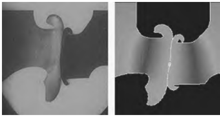
Fig. 74 Comparison of actual (left) with predicted (right) weld shape during the inertia welding of two dissimilar materials, as would occur in a compressor spool with two adjacent stages made of different materials. Due to differing material characteristics on the two sides of the weld interface, modeling is crucial in determining the right weld geometry and parameters. Source: Ref 33
