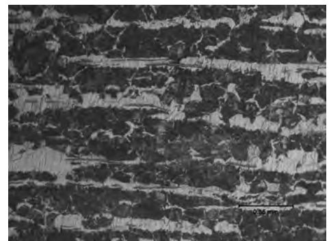
Fig. 48 Micrograph showing banded structure of medium-carbon steel and presence of inclusions. Original width of image is 0.3 mm.
