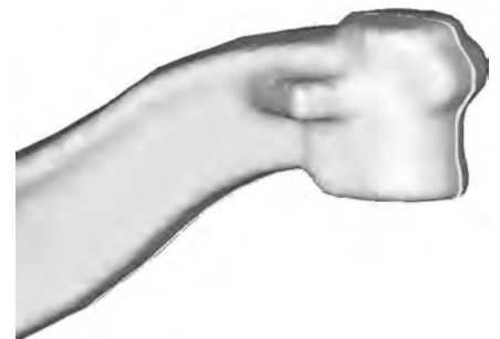
Fig. 25 The as-forged shape is shown in the front (lighter color), with the heat treated shape behind (sliced and darker color). The phase transformation was the key reason for this distortion
