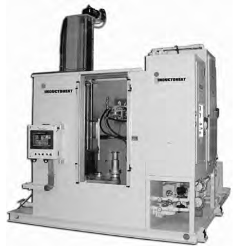
Fig. 76 Inductoheat's single-coil dual-frequency system comprises medium-frequency (10 kHz) and high-frequency (120 to 400 kHz) modules working simultaneously or in any sequence desirable to optimize properties of induction heat treated gearlike components. Total power exceeds 1200 kW. Source: Ref 28
