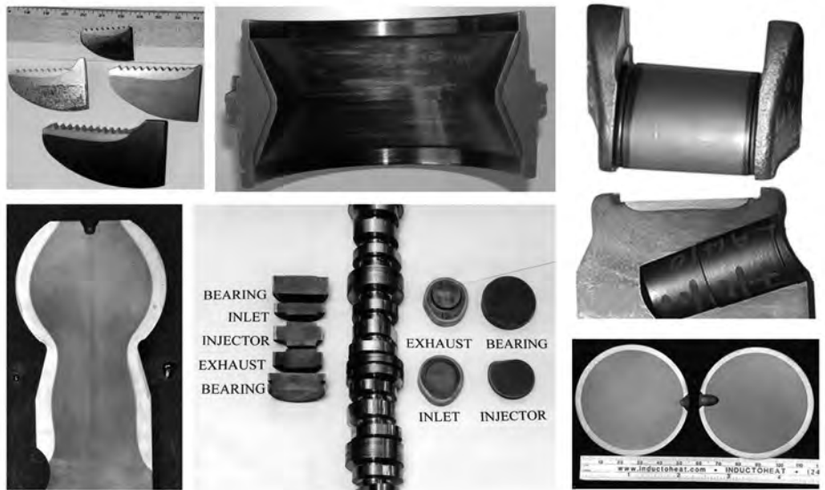
Fig. 3 Various applications and part geometries that require specific hardness profiles. Courtesy of Inductoheat, Inc.
