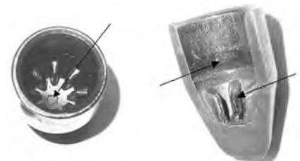
Fig. 30 Arrows highlight the defects observed after forming the electrode
