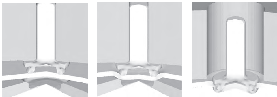
Fig. 63 Installation of the drawform stud. The plastic strain is shown as the shaded color
