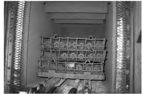
Fig. 35 Arrangement of load in tempering furnace
