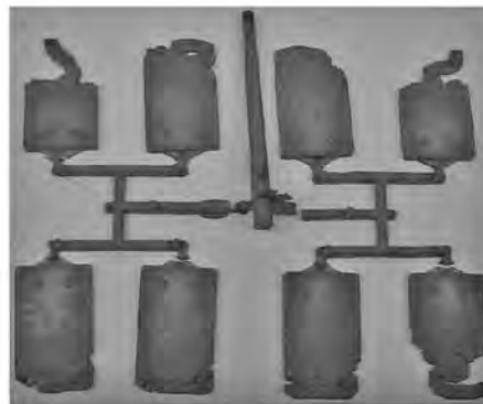
Fig. 10 (a) Finite-element modeling mesh for a multicavity and delivery system. (b) Filling experiment showing the different filling pattern by changing the filling time ( t_f ) from 4.0 to 0.5 s. Source: Ref 26
