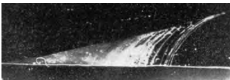
Fig. 24 Traces of a moving boundary in a zinc bicrystal (reversed-capillary technique). Source: Ref 2
