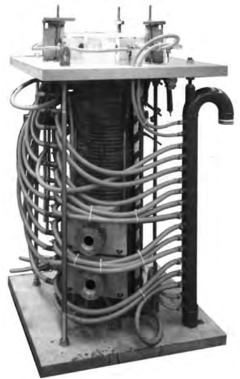
Fig. 62 Vertical inductor for static heating of large billets. Courtesy of IHWT, United Kingdom
