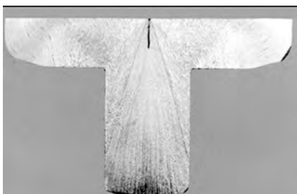
Fig. 37 Pressure valve extrusion showing pipe-type defect in the center
