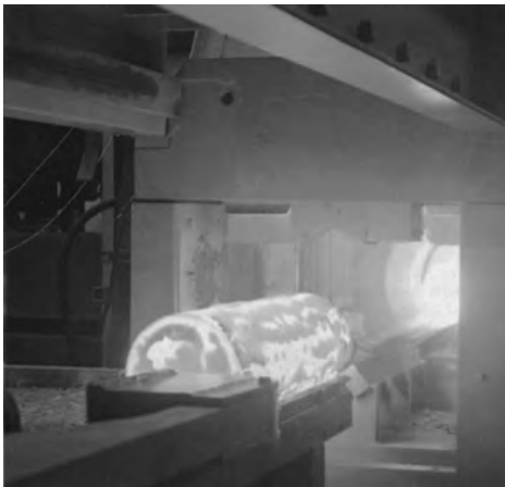
Fig. 59 Progressive multistage horizontal heating of large steel billets. Courtesy of Inductoheat, Inc.
