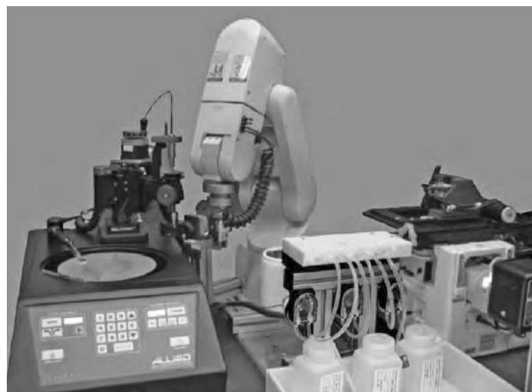
Fig. 11 Major components of Robo-Met.3D system: automatic polisher (left), robot arm (center), automatic etching station (lower center), and motorized inverted microscope (right). Source: Ref 15
