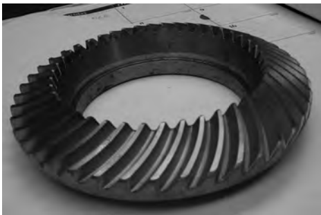
Fig. 69 Bevel gear shape increases complexity of model
