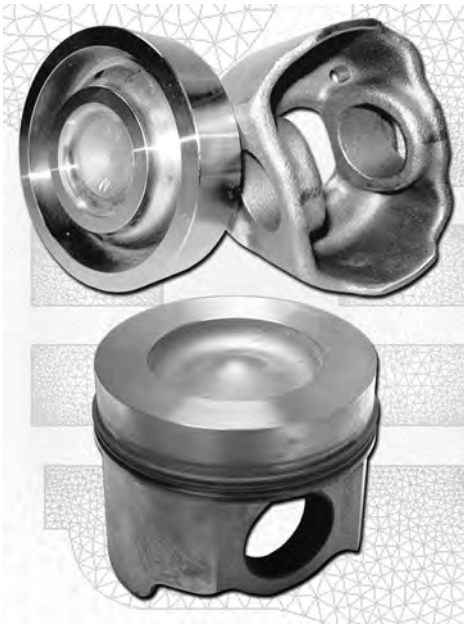
Fig. 38 The Monosteel piston starts out as two separate forgings. Source: Ref 29
