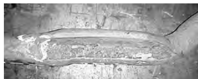
Fig. 24 Once the fold location was established from simulation, the defect was identified on the actual axle beam after bending (location shown by chalk)
