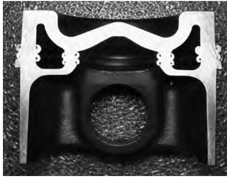
Fig. 39 Cross section of a friction-welded piston. Source: Ref 29
