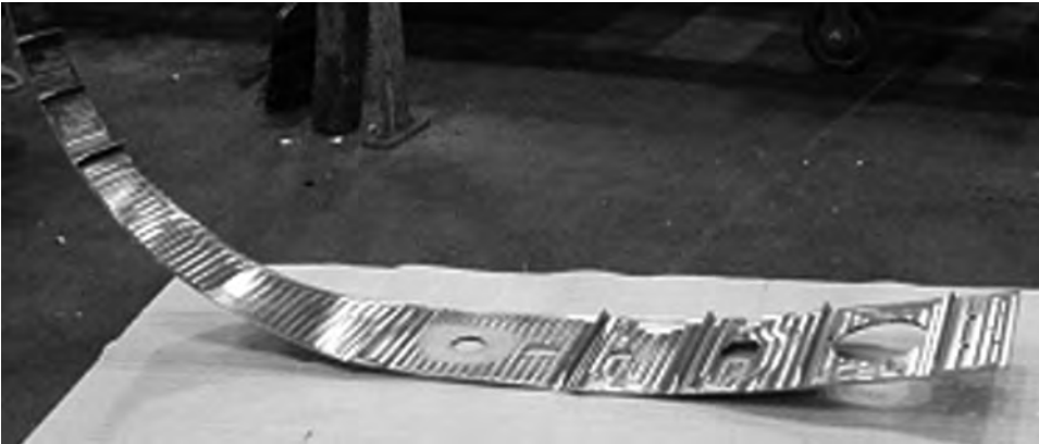
Fig. 5 Distorted airframe component. This component was machined flat. The material stress and machining-induced stress are causing it to distort
